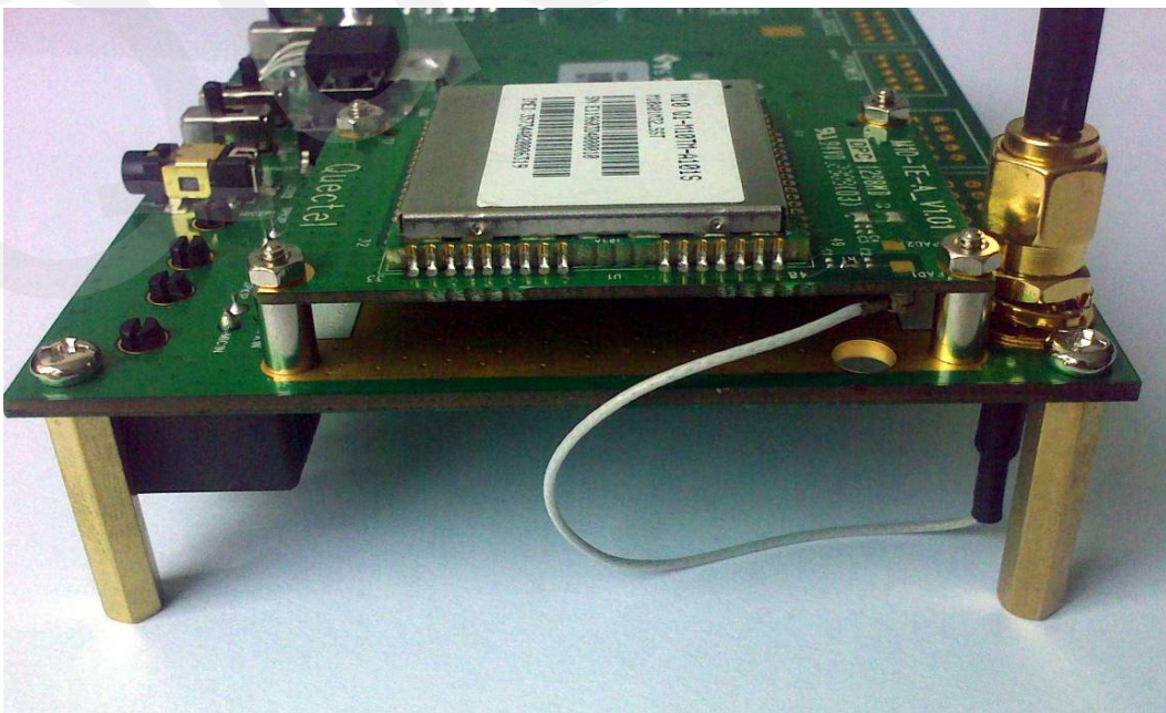
Figure 17: Bolts to support EVB
